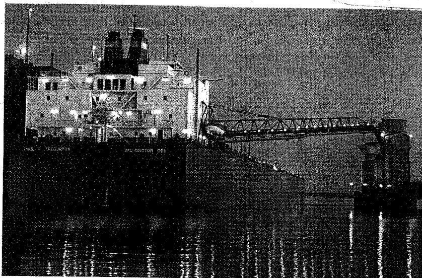
The Paul R. Tregurtha discharges coal in Marquette, Mich. The vessel, with an overall length of 1,013.5 feet, is the largest ever built for the Great Lakes trade.
